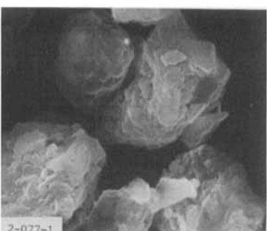
FIGURE 4. SEM images of individual coal particles (top row) and coal microagglomerates (bottom two rows) produced by oil agglomeration and extraction with hexane. Pittsburgh No. 8 coal on the left, Upper Freeport coal on the right.
